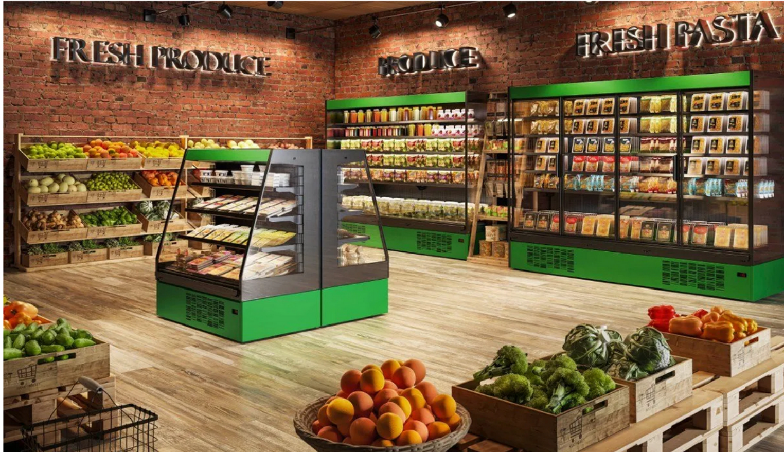
Epta's new Spices range of R290 plug-in cases includes an open semi-vertical (Pepper), an open vertical (Ginger) and a closed vertical (Vanilla). (Source: Epta)
